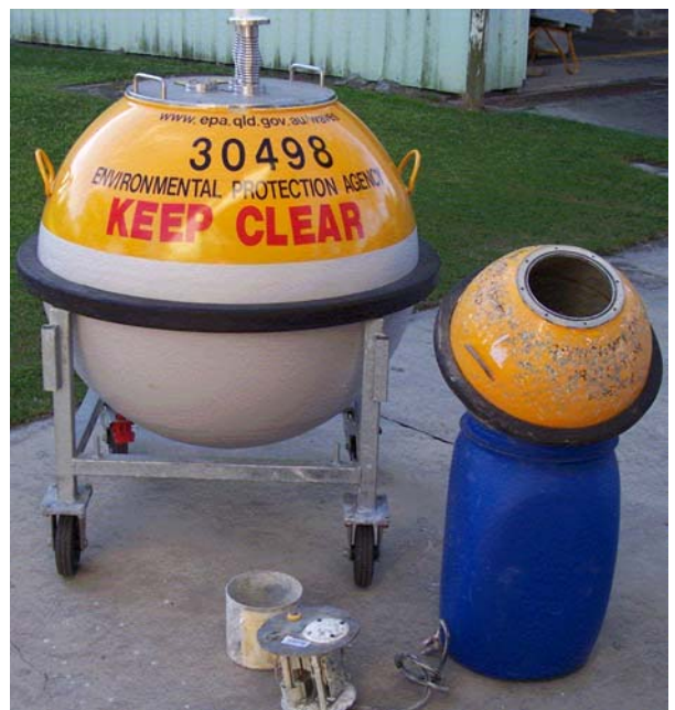
Figure 4 – Damaged BOB beside moored wave buoy
