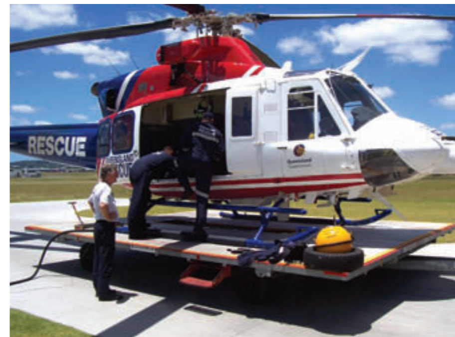
Figure 5. Using a helicopter to deploy the DWR-G4 in the path of a tropical cyclone [4]. Picture courtesy of EPA
