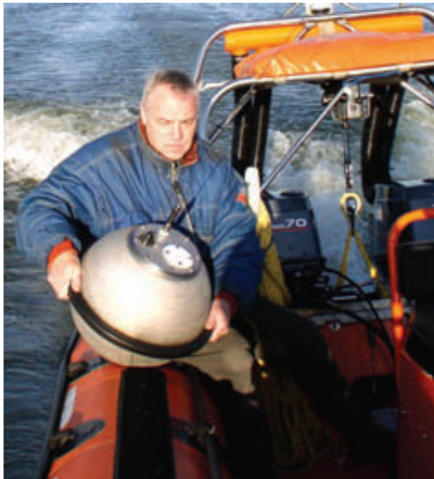
Figure 1. The small GPS-based directional wave buoy (DWR-G4) can be deployed by hand
