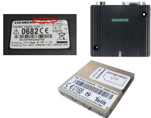
Photographs of earlier Siemens and later Telit GSM modems used in Waverider buoys.
