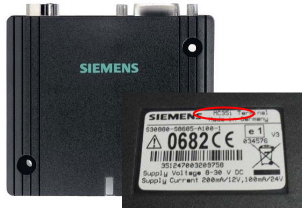
Photographs of Telit and Siemens GSM modems used in Waverider buoys. As for the Siemens modem the particular model is critical. Check the label on the bottom side (area inside red ellipse).
